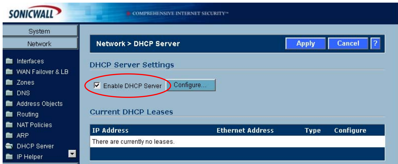
Screenshot 1: Enabling the internal DHCP server
